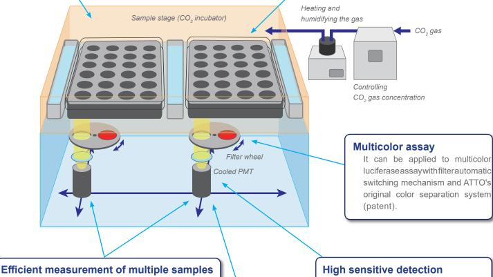
Since two plates are scanned simultaneously by two detectors, more samples can be measured at shorter intervals.
